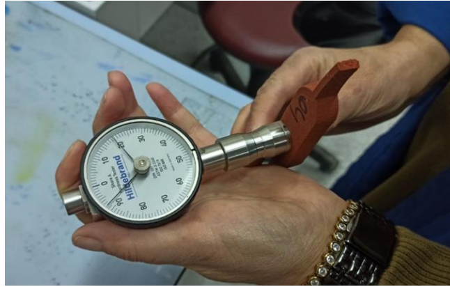
Figure 4-4. Hand-held analog durometer type A.
