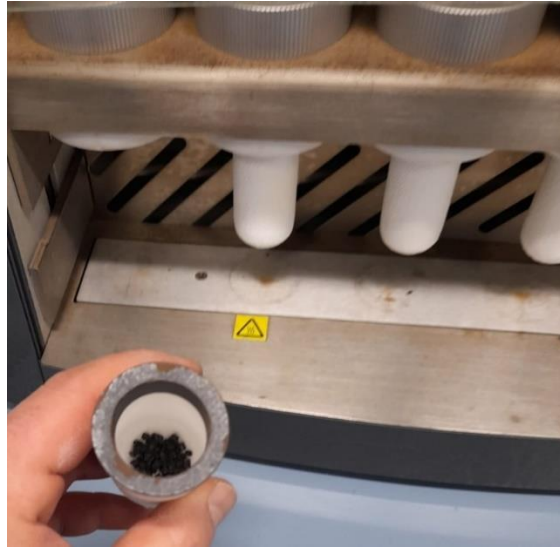
Figure 4-6. A photo of soluble fraction test samples before extraction.
