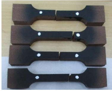
Figure 4-2. A photo of dog-bone shaped samples after uniaxial tests were completed.
